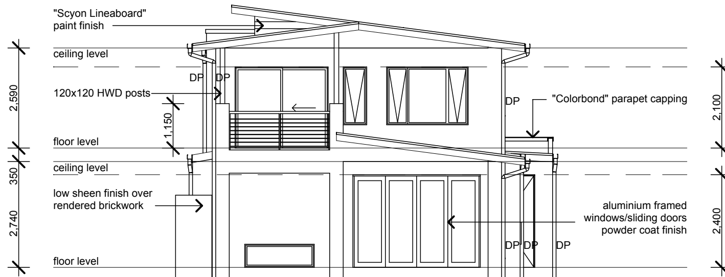
NORTHERN ELEVATION SCALE 1 : 100
