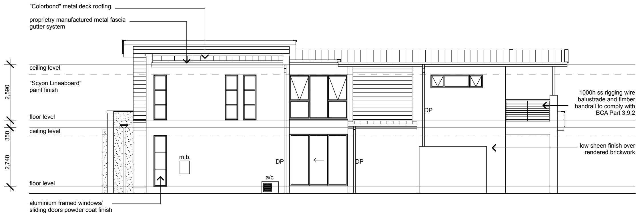
EASTERN ELEVATION SCALE 1 : 100
